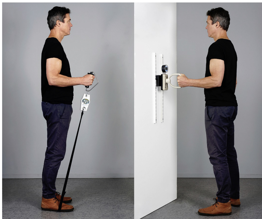
FIGURE 1: Test of lifting strength and forearm torque.
